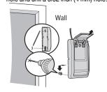
1.4 Install the bottom screw, allowing 1/8 inch (3 mm) to protrude from the wall.
